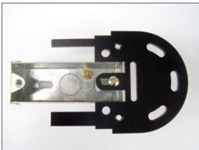
The base end cap plate is first held in position on to the architrave back box through either of the slots in the plate. One slot allows longitudinal movement the other horizontal if fitting to paired box ends. As above, once the end cap plate is held in position on the architrave box the wall can be marked for drilling. Remove plate to enable drilling and plugging. Proceed with the wiring and cover plate fitting as in No1
